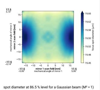
spot diameter at 86.5 % level for a Gaussian beam ( $M^2 = 1$ ) with 10.0 mm diameter at  $1/e^2$ , clipped at 10.0 mm field size and mirror distances as given above for a two mirror scan system
